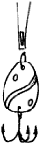
Lure made from a thrift store spoon: cut off the handle and file smooth.
