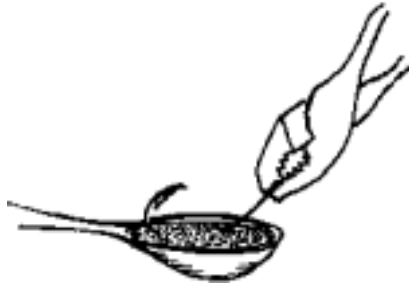
Setting a hook into a cast spoon-mold lure
